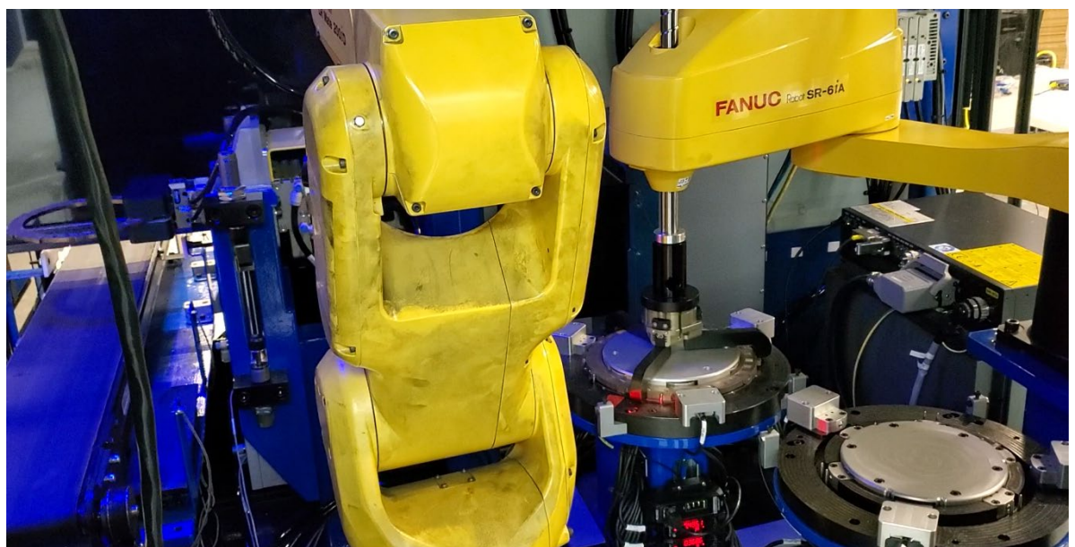
4-axis robot picking part from one of the gages
