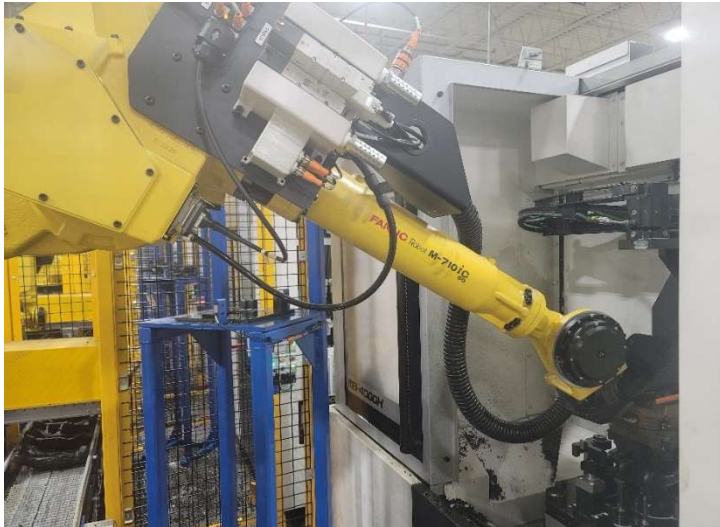
6-axis robot loading a part into CNC machine
